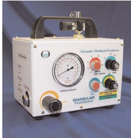
The Magellan ventilator features a pneumatic control system. It's simpler than electronic controls and is more dependable in harsh environments.
